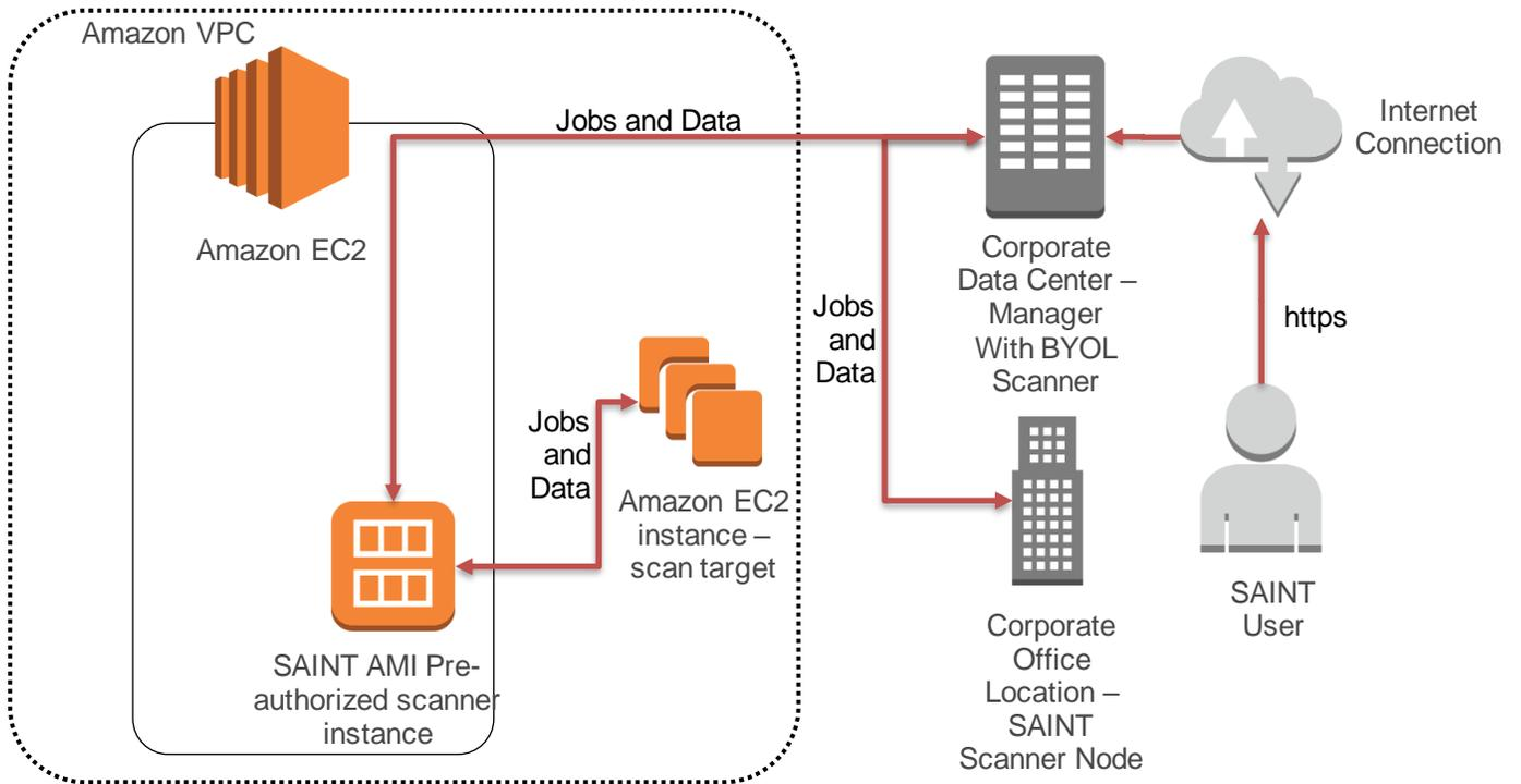
Figure 3 – Hybrid SAINT AMI and External SAINT manager Deployment
