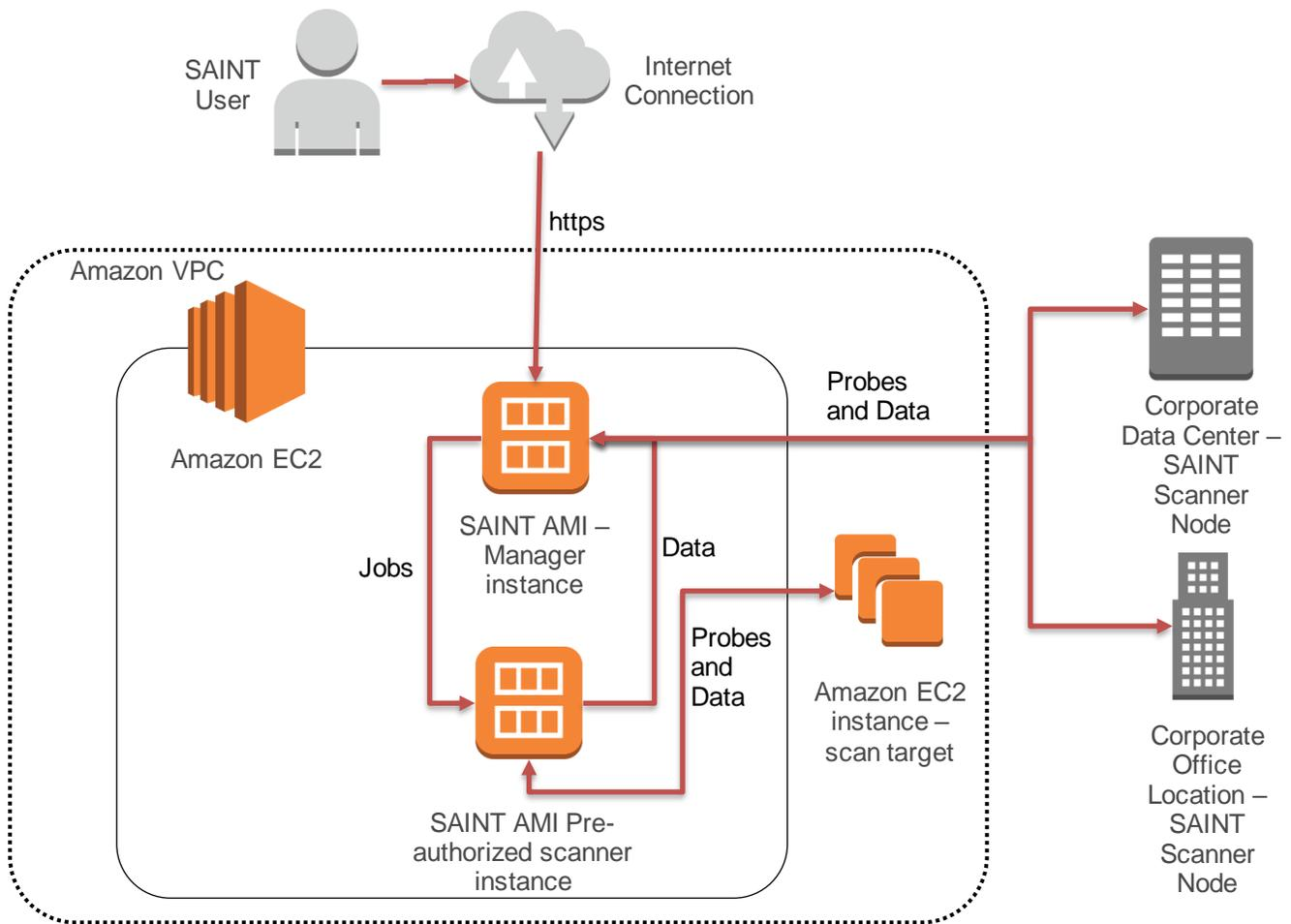
Figure 2 – Hybrid SAINT AMI and External AWS Deployment
