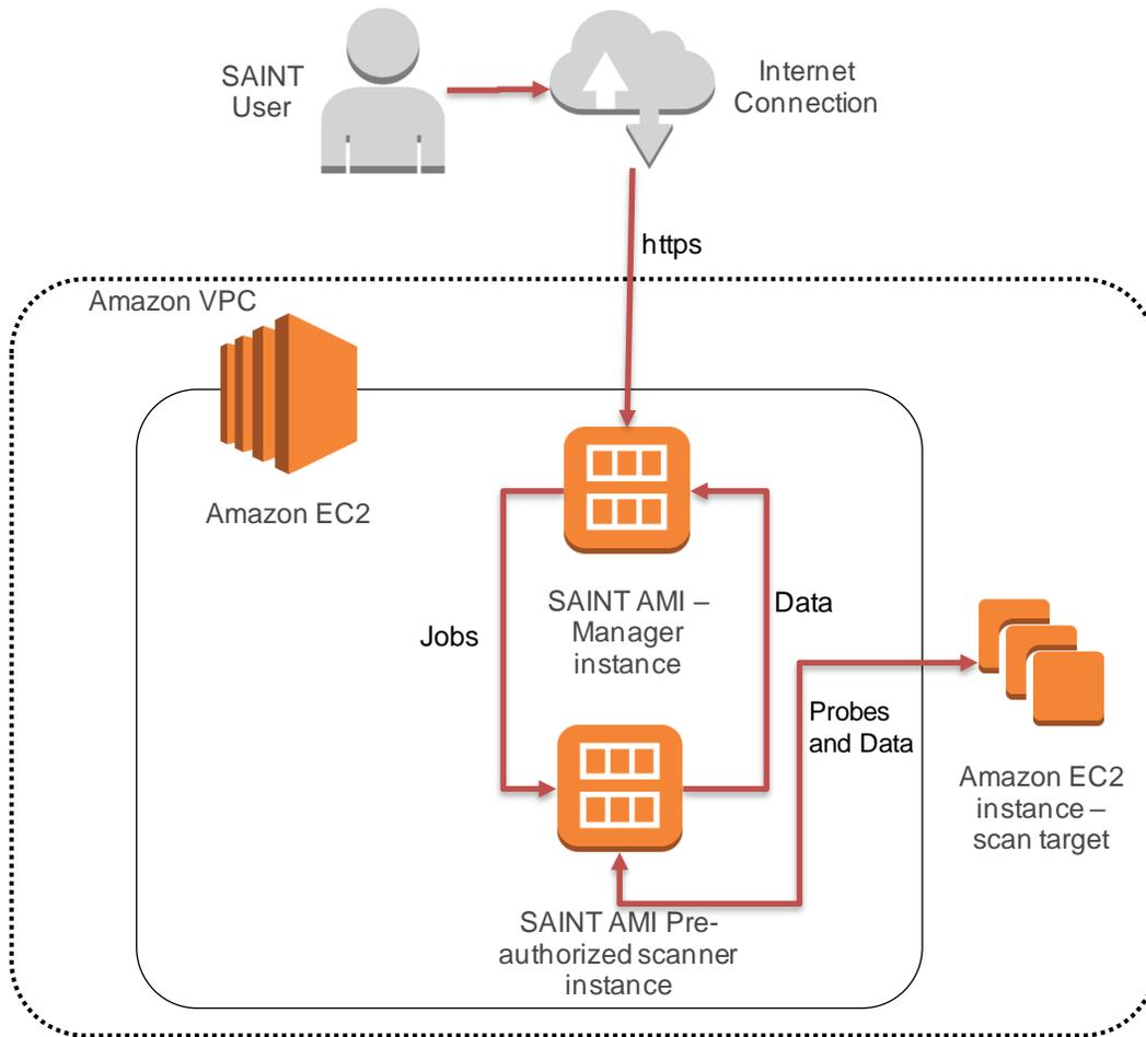
Figure 1 – Standard SAINT AMI Deployment
